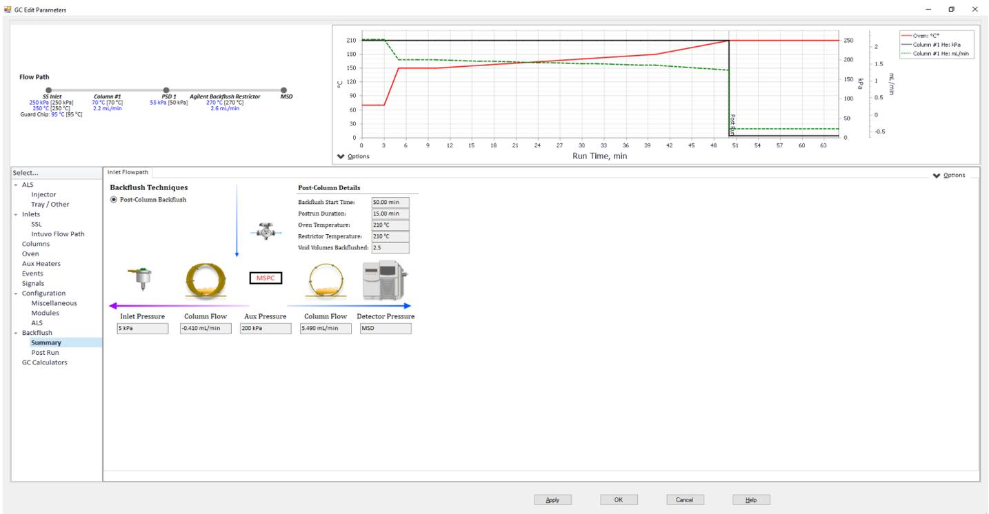
Figure 1. Screenshot of backflush calculator in Agilent MassHunter Acquisition software.
