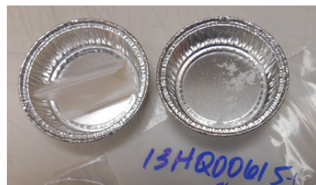
Figure 4A. Seized sample of powdered cocaine, which was sampled using a pocket tip probe. The probe was then placed against a piece of clean weigh paper, pocket tip facing down, and rinsed twice with methanol. Once the probe dried, it was inserted into the probe holder, which was previously cleaned with water and dried with a laboratory wipe.
