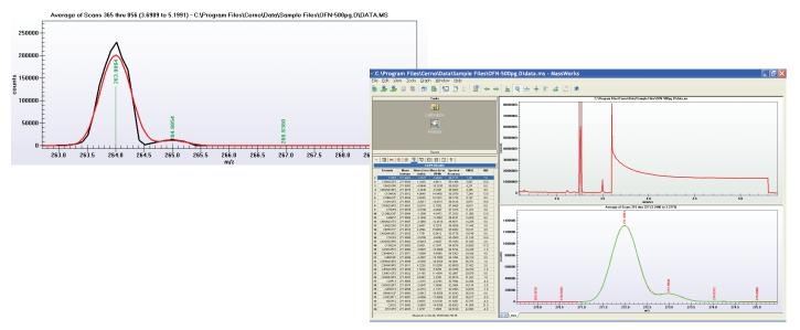
Applying the PFTBA calibration to OFN peak eluted at 3.25 minutes. The accurate monoisotope mass of OFN is found within 2 mDa of its exact mass. CLIPS elemental composition search correctly identifies its elemental composition with the highest spectral accuracy of 99.7% where its theoretical (green) and calibrated (red) mass spectrum is matched down to noise level.
