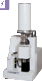
Measurement of Contraction Behavior of Separators by TMA
