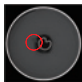
18650-Type Lithium-Ion Battery - Deteriorated Battery CT Image
