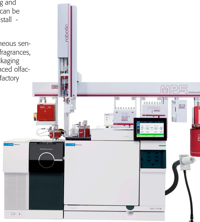
GC/MS System equipped with GERSTEL MultiPurpose Sampler with Dynamic Headspace (DHS) and a GERSTEL Thermal Desorption Unit (TDU) as well as the GERSTEL ODP. The system is an optimized solution for flavor analysis and for concentration and determination of trace level odors.
