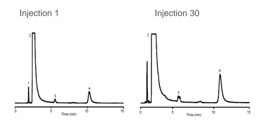
Column: StableBond SB-C8, 4.6 x 150 mm, 5 mm Mobile Phase: 60% 25 mM Na<sub>2</sub>HPO<sub>4</sub>, pH 3.0 : 40% MeOH Flow Rate: 1.0 mL/min Temperature: 35°C Detection: UV 254 nm Sample: Filtered OTC Cold Medication: 1. Pseudoephedrine 2. APAP 3. Unknown 4. Chlorpheniramine
