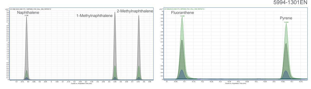
SIM chromatogram of naphthalenes with PDMS fibers (black trace =  $100 \mu m$ ; green trace =  $30 \mu m$ ; blue trace =  $7 \mu m$ )
