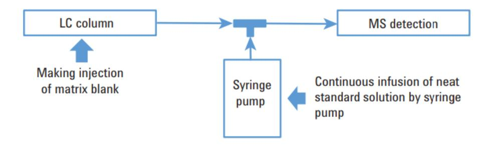
Post column infusion setup for evaluation of ion suppression caused by the matrix
