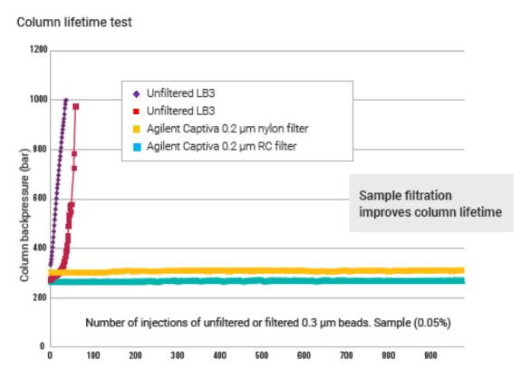
Impact of filtering a 0.3  $\mu m$  latex-bead suspension on lifetime of a sub-2  $\mu m$  column.
