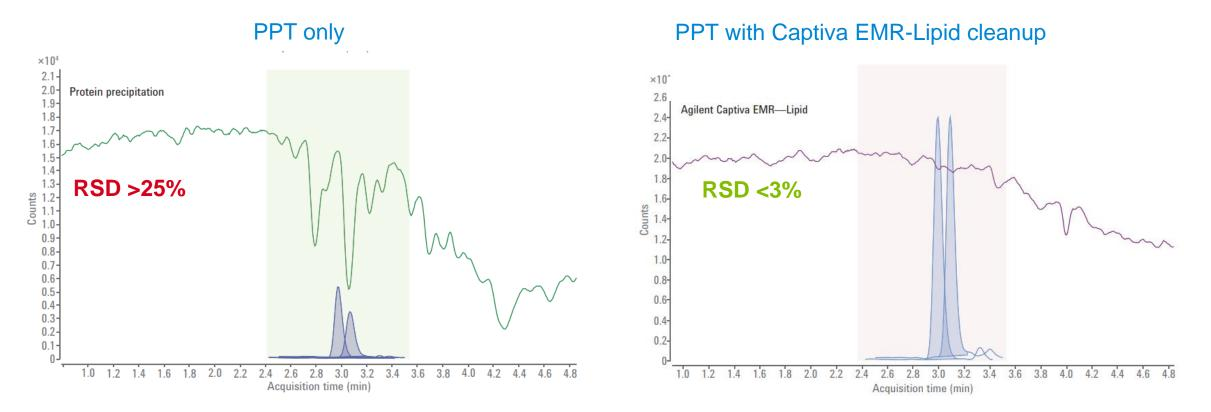
Lipids cause reproducibility problems resulting in high RSD values. Using Captiva EMR-Lipid enables low RSD values and higher peak areas. Higher peak area due to less ion suppression can lead to lower detection limits.
