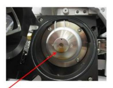
Image shows the build up on the ESI-MS inlet after 3000X urine dilute and shoot injections.
