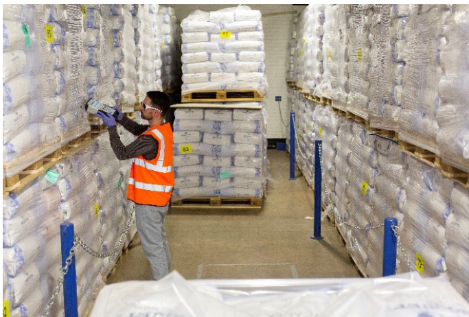
Figure 1. The Agilent Vaya Raman handheld spectrometer being used to measure materials through a paper sack in a quarantine warehouse.
