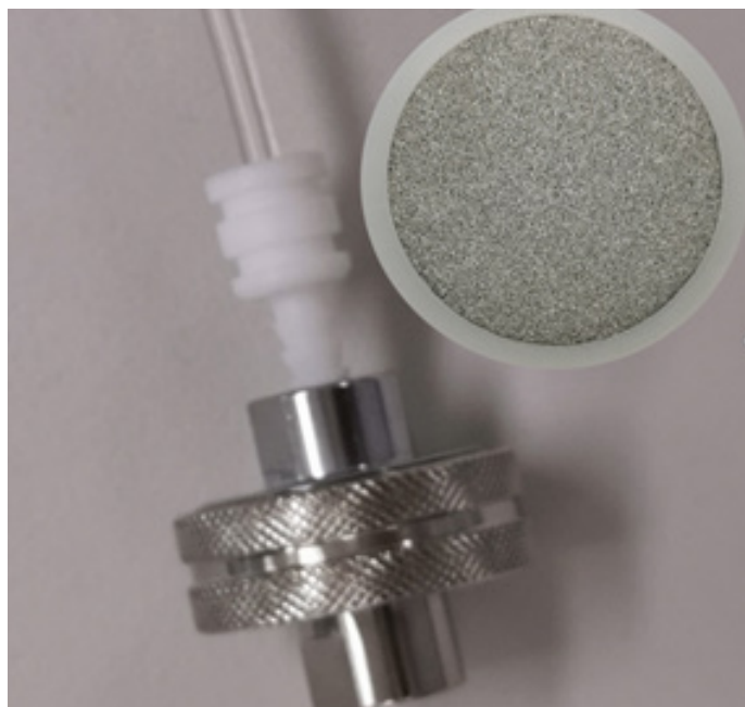
Figure 2. The pre-prep filter disk used to collect the microplastic particles
