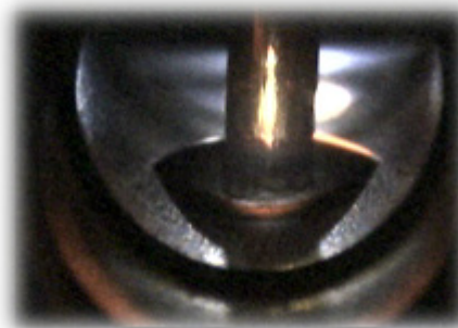
Figure 1. The view inside the tube, using the integrated camera. The probe is dispensing the sample into the tube.
