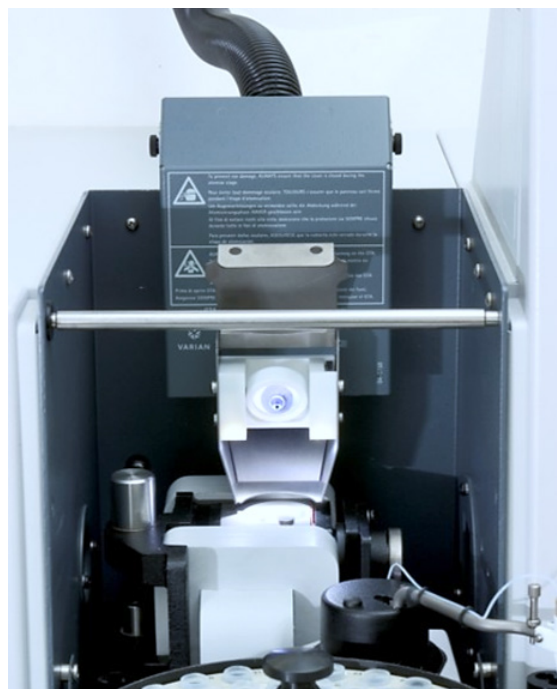
Figure 3. The optional extraction/LED accessory for the Agilent furnace.
