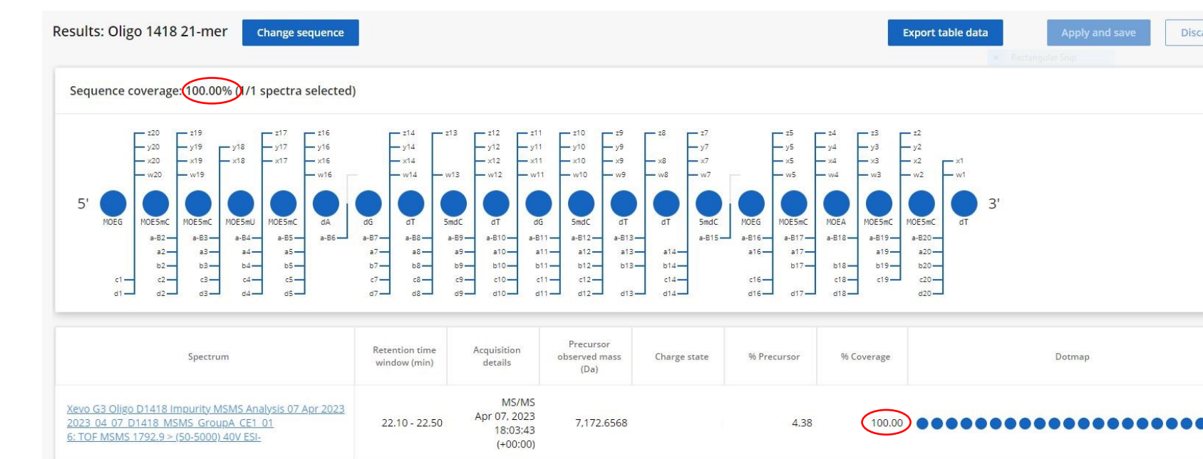
Figure 4. Complete sequence coverage (100%) resulted from the MS/MS fragmentation of the [M-4H] -4 precursor (m/z=1792.14) of the 21-mer siRNA oligonucleotide. The precursor was fragmented with an optimized fixed collision energy (40 V) in the collision cell of a Xevo G3 QToF mass spectrometer.
