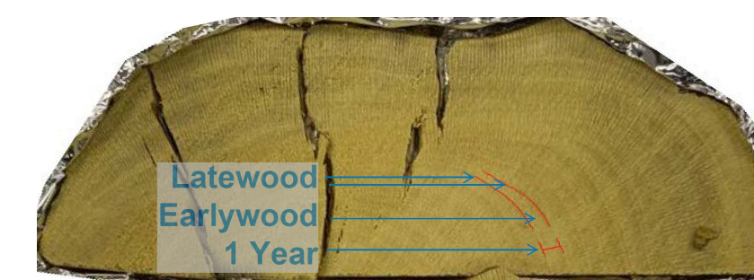
Figure 6. Transverse cross section of French barberry wood
