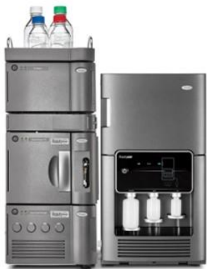
Figure 1: BioAccord™ UPLC-TOF MS System with Max Peak™ High Performance Surfaces. Column used: ACQUITY™ Premier OST Column 1.7 μm, 130 Å, 2.1 x 150 mm More method information can be found in the three application notes listed under the reference.
