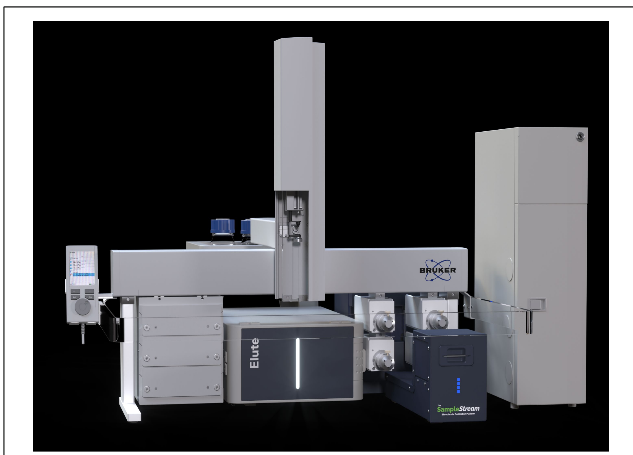
Figure 1. Elute SampleStream. This peripheral can be easily integrated into current mass spectrometry workflows. It can perform various sample preparation steps prior to MS introduction, such as rapid solvent exchange, and/or sample preconcentration. This device was configured to be compatible with a wide range of solvents. Operation is performed all under Hystar, to ensure a seamless workflow transition from sample preparation to mass spectrometry.
