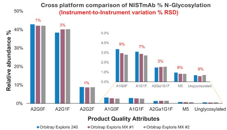
**Cross-platform consistency** demonstrated in the relative abundance measurement of NISTmAb N-glycosylation between Orbitrap Exploris 240 mass spectrometer and Orbitrap Exploris MX mass detector. Data were averaged from 10 replicate injections per instrument. RSDs are <9%.
