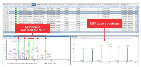
TMT accuracy and precision is enhanced by utilizing TMT SPS MS³ methods and the number of identified peptides is improved with Real-Time Search-Aided methods. Proteome Discoverer software results allow for the visualization of MS² fragment ions that are selected for MS³ and the visualization of the MS³ quantitation spectrum for maximum confidence in results.
