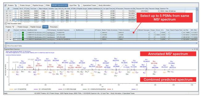
Deconvolution and visualization of chimeric spectra. The experimental and predicted spectrum can be visualized by selecting up to 5 PSMs at a time to display a mirror plot.
