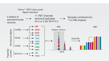
Schematic representation of Pierce TMT11plex Yeast Digest Standard and replicates as an example of study management with Proteome Discoverer software. The standard is composed of four Saccharomyces cerevisiae strains: three lines respectively lacking the non-essential proteins Met6, His4, or Ura2, and the parental strain BY4741 for reference.
