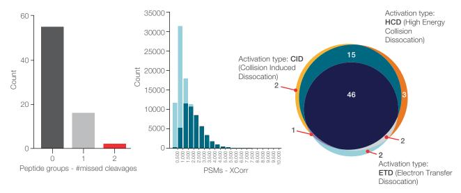
Distribution charts can be utilized to visualize, interpret, and optimize experimental procedures, data acquisition settings, and results. For example, a bar graph can display the number of missed cleavages, a histogram can show the Xcorr values for PSMs passing the pre-set FDR filter (dark red) and excluded hits (salmon), and Venn diagrams can display peptide sequences identified by different fragmentation techniques.
