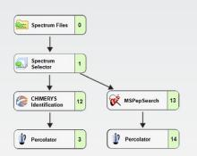
The flexible workflows of Proteome Discoverer software allows for search engines to be used independently, in series, or in parallel to significantly increase the number of peptide and protein identifications.
