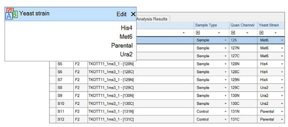
Proteome Discoverer software enables the creation and mapping of sample types, study factors, and quantification channels to data files for simplified and integrated study management.
