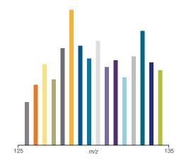
Selecting only identified fragments for the MS<sup>3</sup> event and excluding the ions that either do not carry the TMT tags (y-ions in this case) or that do not belong to the identified peptide increases the signal-tonoise ratio of the reporter ions and significantly improves the throughput and quantitative accuracy of the experiment (right).
