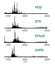
Representative MS<sup>2</sup> spectra of the 27+ parent ion. The spectra were obtained by multiple fragmentation techniques and showed different fragment ion patterns, providing complementary information and increasing the primary amino acid sequence coverage for this protein.
