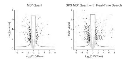
TMT analysis of two cell types revealed more differentially expressed proteins when using SPS MS<sup>3</sup> with Real-Time Search compared to the MS<sup>2</sup>-based experiment. The MS<sup>3</sup> experiment allows for more accurate quantitation, enabling detection of subtle changes in more proteins for each individual cell.
