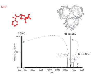
$MS^3$ -based isolation and activation of the intact membrane protein-ligand assembly promote the release of the ligand (*m/z* 350.0). This singly-charged ion is isolated (gray bar) for  $MS^4$  step to allow full structural characterization. (Note: in this experiment the ligand at *m/z* 350.0 was detected in the ion trap. Both the Orbitrap and the linear ion trap mass analyzers can be used to detect ions across the entire *m/z* range).
