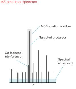
When analyzing complex peptide mixtures, coisolated ion interferences can occur despite using narrow precursor isolation. Co-fragmentation of precursors of interest and interfering ions negatively impacts the quantitative accuracy of the TMT-based experiment.\*
