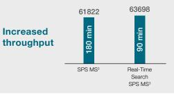
Real-Time Search directs the mass spectrometer to perform MS<sup>3</sup> only on identified precursors. As a result, it doubles the throughput of SPS MS<sup>3</sup> experiments. Shown here are data for an HHM sample: three human cell lines labeled as biological replicates in 10plex (3-3-4). (*Data courtesy Devin Schweppe and Qing Yu, Harvard Medical School*)
