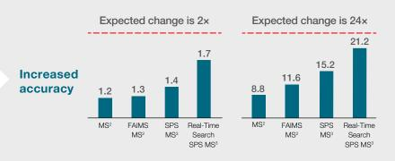
For each TMT channel, 4–100 pmol of a six-protein digest was added to 40 µg of HeLa digest, and then labeled, resulting in a spiked-in standard mixed in ratios of 2–24 (2, 4, 8, 12, 16 and 24). Only combined averages for the expected ratios of 2 and 24 are shown here. Higher accuracy afforded by Real-Time Search is indispensable for teasing out subtle differences in protein abundances, including when sub-classifying individual cells (pp 6–7).
