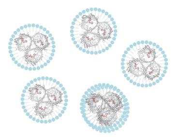
Intact protein complexes are extracted from the membrane using detergent. Detergent molecules form a micelle layer around the protein complex that allows solubilization. The micelles are then ionized using nESI and introduced into the mass spectrometer.
