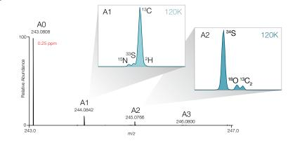
Biotin at 120K resolving power. A1 and A2 isotope fine structure (<sup>15</sup>C, <sup>15</sup>N, <sup>18</sup>O, <sup>33</sup>S and <sup>34</sup>S).
