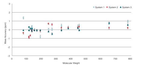
Analysis of 25 components using the optional Thermo Scientific<sup>™</sup> EASY-IC<sup>™</sup> ion source with internal calibration. Independent of molecular weight, all standards (MW 75–776) were measured with excellent mass accuracy over six days on three different Orbitrap Exploris 240 mass spectrometer systems.
