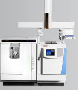
Orbitrap Exploris GC 240 mass spectrometer with the Thermo Scientific<sup>™</sup> TriPlus<sup>™</sup> RSH autosampler
