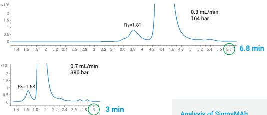
Size exclusion chromatograms of SigmaMAb using an Agilent AdvanceBio SEC 200 Å 1.9 μm 4.6 x 150 mm column.
