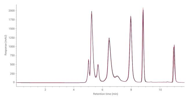
Overlay of eight Bio-Rad protein standard chromatograms for 400 injections at an interval of 50 runs.
