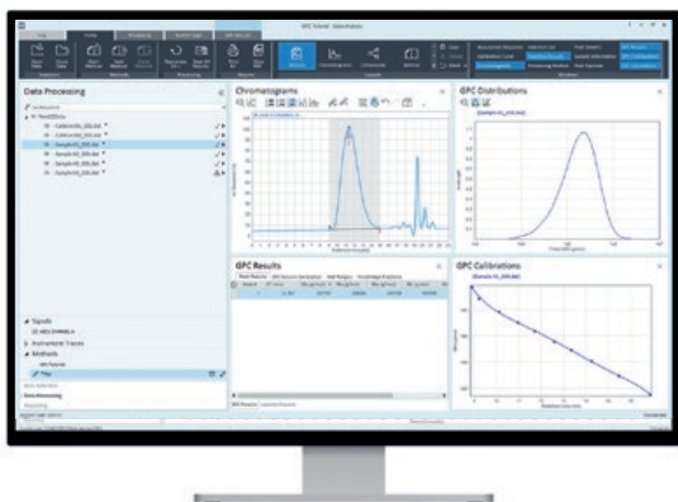
Screenshot of the GPC/SEC software for OpenLab CDS showing the chromatogram and molecular weight distribution for a polystyrene sample.
