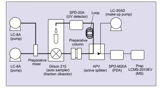
Fig.1 Flow Diagram of Preparative LC-MS System
