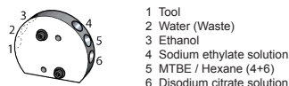
Figure 5: Up to 5 different solvents and solutions may be dispensed by the dilutor tool.
