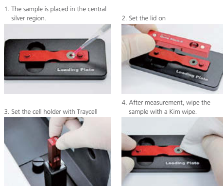
Figure 2 What the Nano Stick Looks Like and How To Use It
