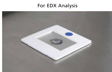
For EDX Analysis Close the EDXIR-Holder and face the polypropylene film towards the irradiated side (facing down)
