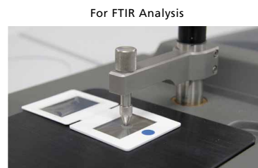
For FTIR Analysis Open the EDXIR-Holder and push the sample adhered to the adhesive film up against the prism.
