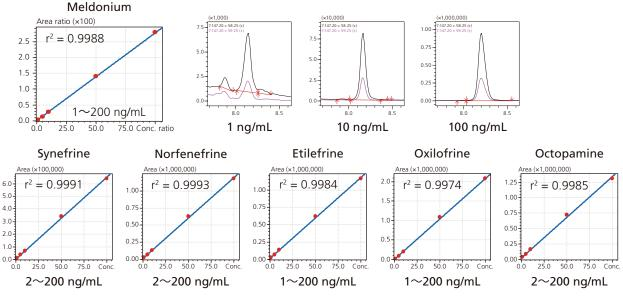
Fig. 4 Calibration Curves and MRM Chromatograms of 6 Compounds
