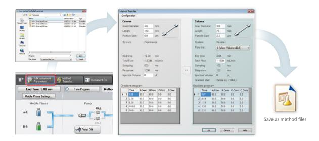
The i-Series MT system has two flow lines matched to the UHPLC and HPLC delay volumes. In addition to simplifying method transfer for customers using HPLC, this single integrated system also streamlines reviewing procedures for increasing the speed of customers' methods using UHPLC.
