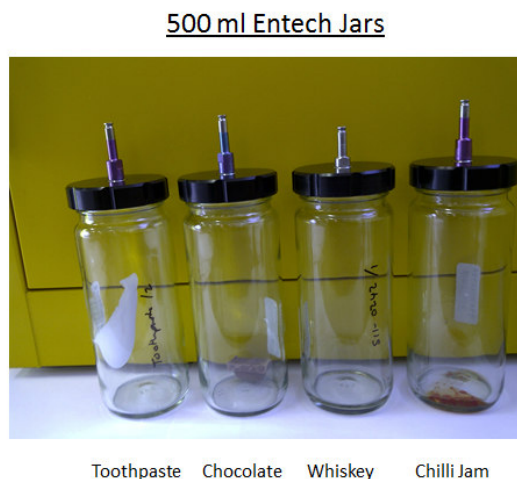
Figure 1 Water based products in Entech Large Volume Headspace jars (2g Toothpaste, 10 g Chocolate, 5 ml Whiskey, and 1 g of Chilli Jam).
