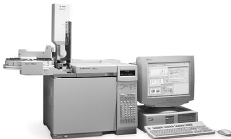
Fig 1: GC 6890 with autosampler
