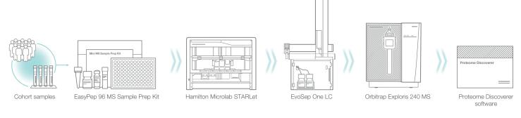
Ultra-high throughput plasma protein profiling (uHTPPP) workflow using the Thermo Scientific™ Orbitrap Exploris™ 240 mass spectrometer.
