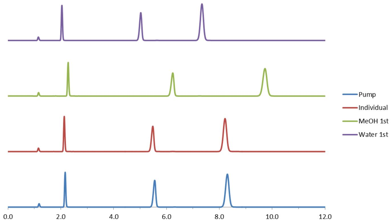
*Kinetex™ 5μm XB-C18 150 x 4.6mm; 60:40 MeOH: H2O
