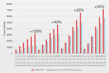
performance across different protein loads and run times (Figure 3). In particular, CHIMERYS enables considerable improvements over traditional search algorithms for shorter gradients and higher protein loads. This enhancement enables more efficient data acquisition schemes for increased sample throughput and instrument utilization.
