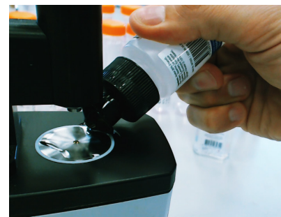
Figure 3. The neat hand sanitizer sample is placed onto the ATR accessory, fitted to the Cary 630 FTIR. The Agilent MicroLab software uses picture-guided workflows to help users to follow each step of the measurement including cleaning and sampling.
