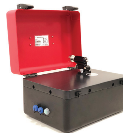
Figure 2. The Agilent 4500 FTIR is a rugged battery-powered portable analyzer, ideal for analysis in the field.
