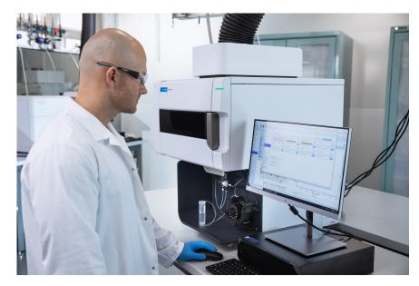
The Agilent 5800 ICP-OES does not require any flammable gases and is safe to run unattended and in remote locations.
