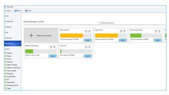
The early maintenance feedback function of Agilent ICP-0ES instruments tracks instrument use and alerts the operator when maintenance tasks are required.
