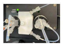
The SampleSense dual sampling valve, installed on an Agilent ICP-OES instrument The valve is available in a variety of configurations.
