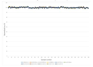
240 samples were analyzed in approximately 30 minutes using an Agilent 5800 ICP-OES, fitted with a SampleSense valve. All %RSD were less than 1.1% and a measurment time per sample of less than 8 seconds was achieved.
