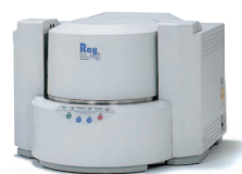
Fig. 5 Photograph of EDX-800HS Energy Dispersive X-Ray Fluorescence Spectrometer
