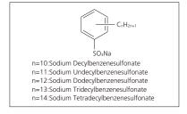
Fig. 1 Structure of Anionic Surfactants
