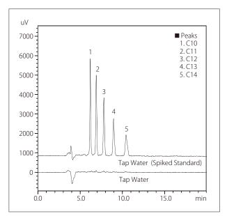
Fig. 5 Chromatograms of Tap Water (20 μL Inj.) (Using Column 2) Upper: Water, 0.04 mg/L each, total 0.2 mg/L spiked Lower: Water
