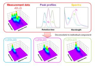
Fig. 3 Peak Deconvolution Process by i-PDeA II
