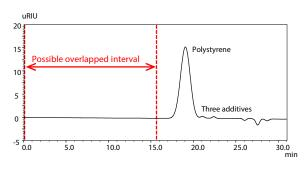
Fig. 1 Chromatogram of Polystyrene and Three Additives (RID)
