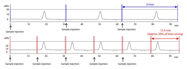
Fig. 2 Comparison of Sequential GPC Analyses With (Lower) / Without (Upper) Overlapped Injection (RID)
