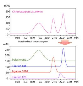
Fig. 5 Deconvolution Result of Three Polymer Additives (PDA)
