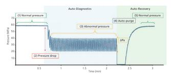
Fig. 7 Diagram of Auto-Diagnostics and Auto-Recovery Functions
