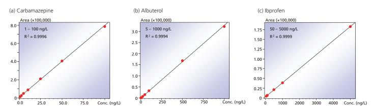
Fig. 2 Calibration curves for Carbamazepine (a), Albeterol (b) and Ibprofen (c); (a) was spiked in river water, (b) and (c) were spiked in lake water.
