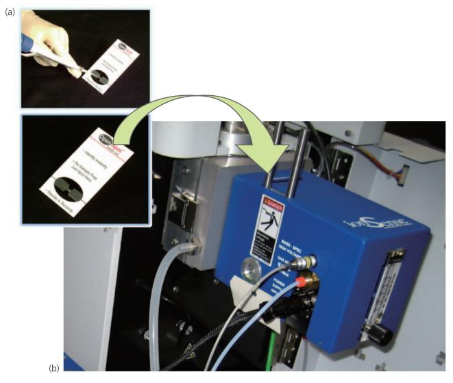
Fig. 2 DART-ID CUBE ion source & LCMS-2020
