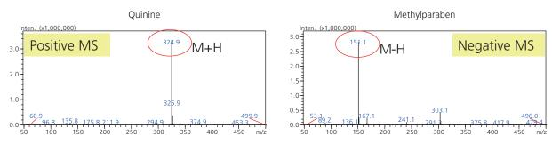
Fig. 3 Standard sample MS spectra using DART-ID CUBE
