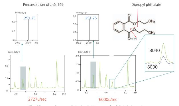
Fig. 6 Precursor ion scan of standard mixture sample of 8 phthalate esters.
