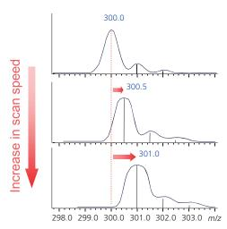
In case of typical triple quadrupole mass spectrometer
