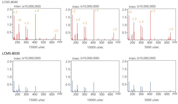
Fig. 5 Q1 scan spectra of pesticides at three different scan speed.
