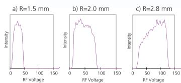
Fig. 2 The optimum operating RF voltage of quadrupole ion guides was acquired experimentally. The voltages were 27 V, 50 V and 100V for R= 1.5, 2.0 and 2.8 respectively.
