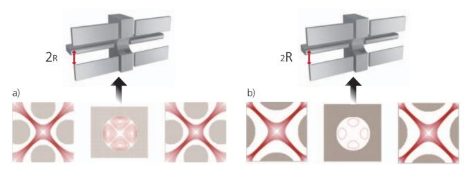
Fig. 4 Simulated fringing focusing field estimates of a) smaller R ion guides was found to be more effective than those of b) larger R. Therefore we have achieved higher sensitivity using smaller R ion guides.
