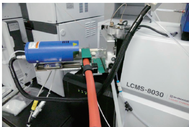
Figure 6 DART-OS ion source with volatile analyzing option & LCMS-8030
