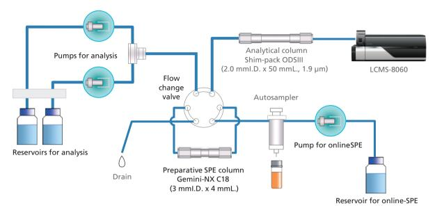
Figure 2. Flow diagram for online SPE system
