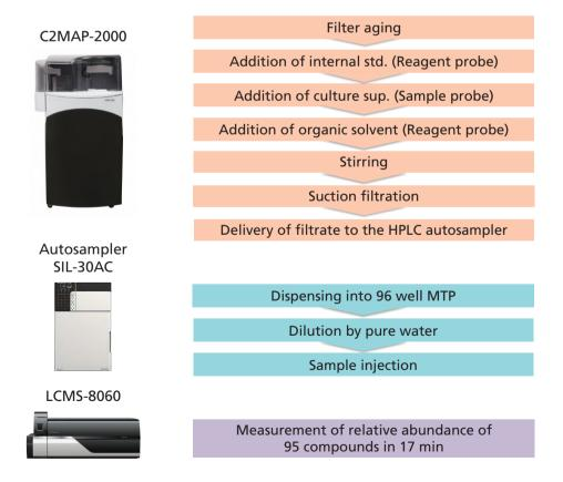
Fig.2 Pretreatment and measurement flow
