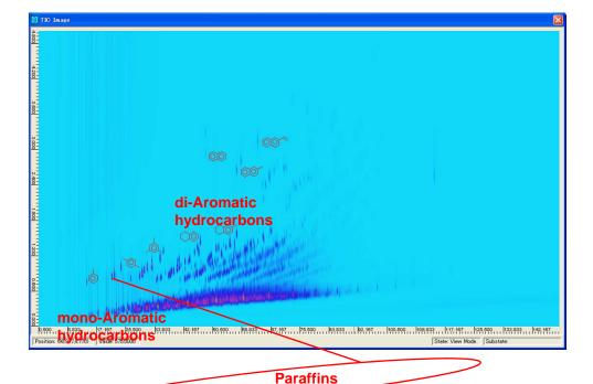
Fig. 1: 2-Dimensional Image of the GC x GC-MS Analysis Results for Kerosene
