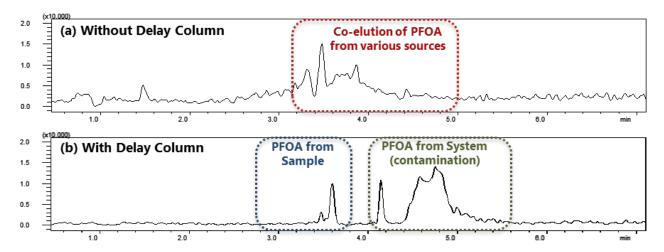
Figure 1. Chromatogram of PFOA: (a) without delay column and (b) with delay column.
