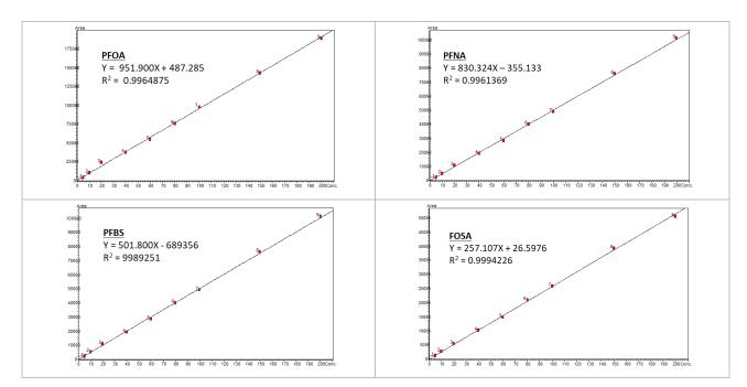
Figure 5. Representative calibration curves (PFOA, PFBS, PFNA and FOSA) at 10 µL injection using LCMS-8060.
