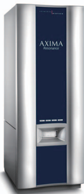
Fig. 7 (a) The Axima Resonance MALDI-QIT-TOF instrument, and (b) its internal configuration consisting of a MALDI Ion Source, Ion Trap, Reflectron and Detector.
