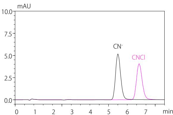
Fig. 2 Chromatogram of Standard Solutions of Cyanide Ion and Cyanogen Chloride (0.01 mg/L each)
