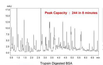
Column : ODS (2.1 mm I.D. x 100 mm, 1.8 µm)
