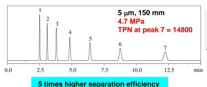
: ODS (4.6 mm l.D. x 150 mm, 5 μm) Mobile Phase: Water/Acetonitrile = 3/7
