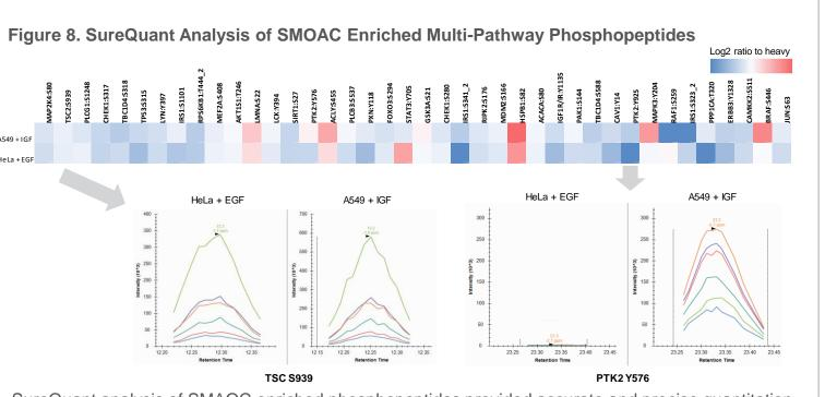
SureQuant analysis of SMAOC enriched phosphopeptides provided accurate and precise quantitation in a single MS run. About 60 light and 134 heavy IS phosphopeptides were quantitated using SureQuant method on Orbitrap Exploris<sup>™</sup> 480.
