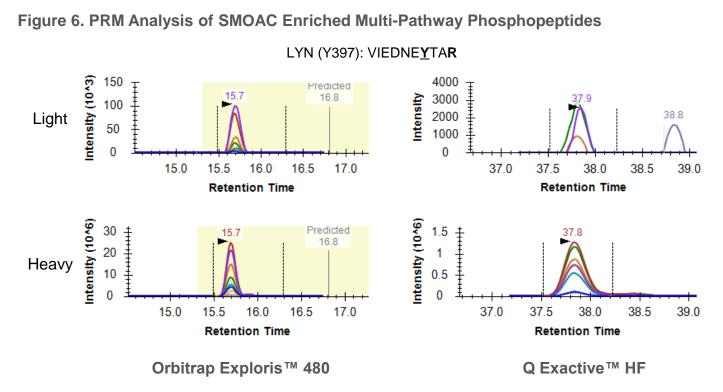
PRM analysis of SMOAC enriched phosphopeptides from A549 (+hIGF) and HeLa (+hEGF) resulted in accurate and precise quantitation of 134 heavy IS phosphopeptides. Improved signal to noise and sensitivity was observed with new Orbitrap Exploris<sup>TM</sup> 480 (Figure 6). Differential expression of many phosphopeptides observed between two cancer cell lines (data not shown).
