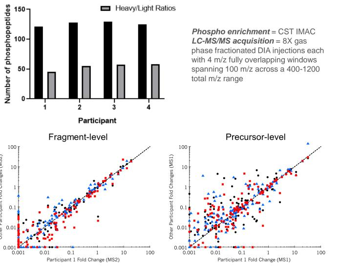
DIA analysis of IMAC enriched phosphopeptides from HeLa (+hEGF) showed better quantitation compared to precursor-level (DDA) analysis. About 50 light and 124 heavy IS phosphopeptides were quantitated across 4 different core labs using standardized DIA workflow (sPRG 2018-2019 study).
