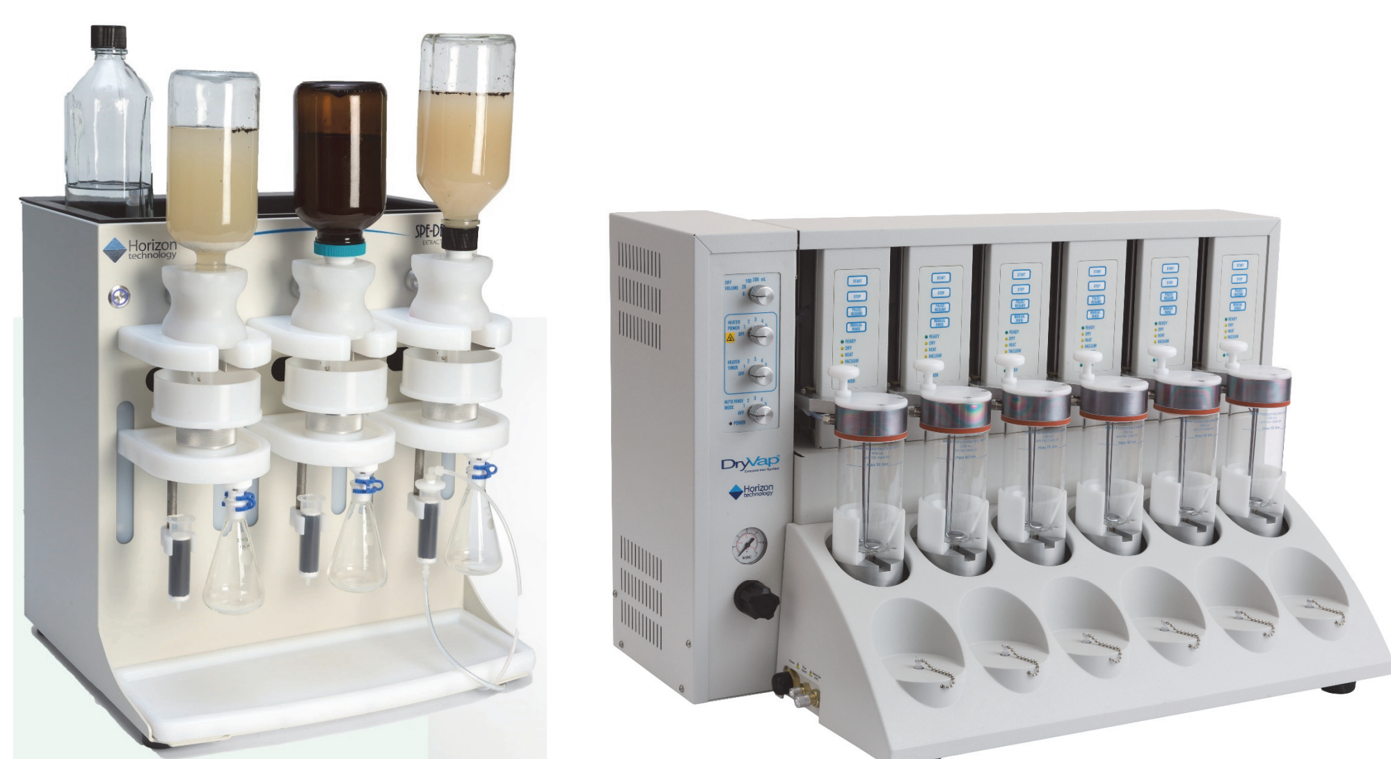
Figure 1. Extraction and drying systems used for sample preparation: the Biotage ® Horizon 5000 (previously known as the SPE-DEX 5000) (left) and the DryVap ® System (right).
